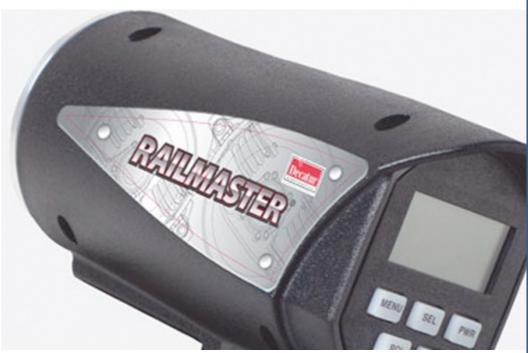
High- and low- speed ranges make the Railmaster the perfect tool for both the marshalling yard and the open track. Mount it on a tripod or pole, or take advantage of its ergonomic grip.
